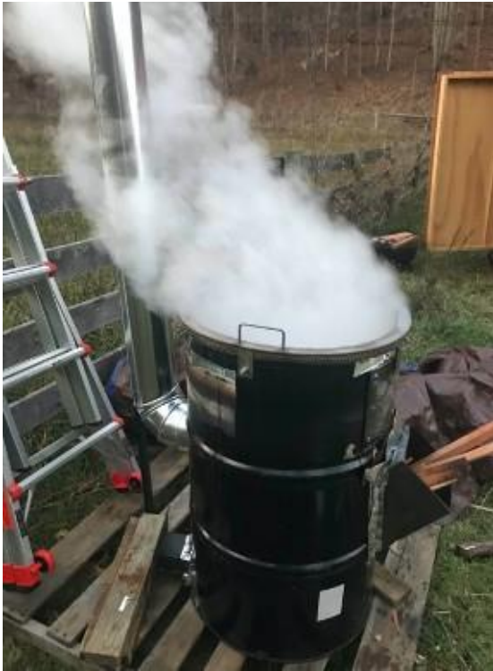
Figure 16 - Rocket Stove Evaporator in action. (Photo Credit: Future Generations University)
