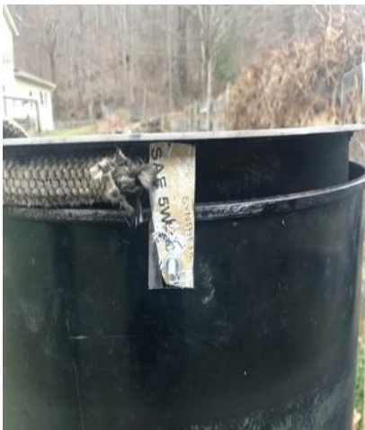
Figure 15 - raised pan with rope gasket. (Photo credit: Future Generations University)
